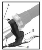
Figure 26- Lever clamp bolt, mountain lever A- Lever clamp bolt
