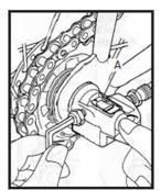
Figure 24- Three-speed bell crank A- Bell crank window
