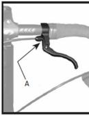
Figure 27- Mid-bar brake lever A- Lever clamp bolt
