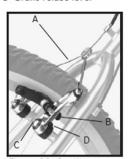
Figure 30- Cantilever brake A- Linkwire B- Pad fixing bolt C- Arm fixing bolt D- Centering screw
