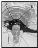
Figure 23- Pulley and cog joint bracket
