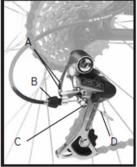
Figure 22- Rear derailleur A- Adjusting screws B- Barrel adjuster C- Cable clamp bolt
