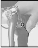
Figure 25- Lever clamp bolt, road lever A- Lever clamp bolt
