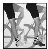
Figure 18- Leg extension with proper seat height
